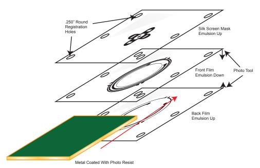
The result is a metal sheet with the protective emulsion removed from the areas which are intended to be etched, while the area which is intended to retain the full metal thickness are protected by the photo resist.
